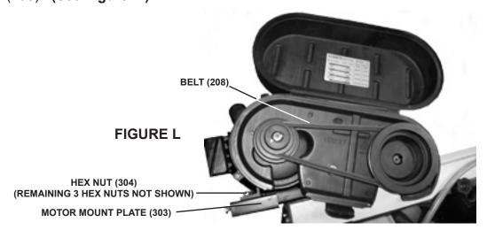
3. Remove the Belt (208) from its two Pulleys (206, 296). Place the Belt onto the two Pulleys according to the Saw Blade (251) speed desired. Then move the Motor (300) back to its original position and secure in place by tightening the previously loosened two nuts and two screws. (See Figures L and M.)
